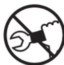
**To avoid damaging the wrench:** Never use the wrench with the power off. Always turn ON the wrench so the applied torque is being measured.
